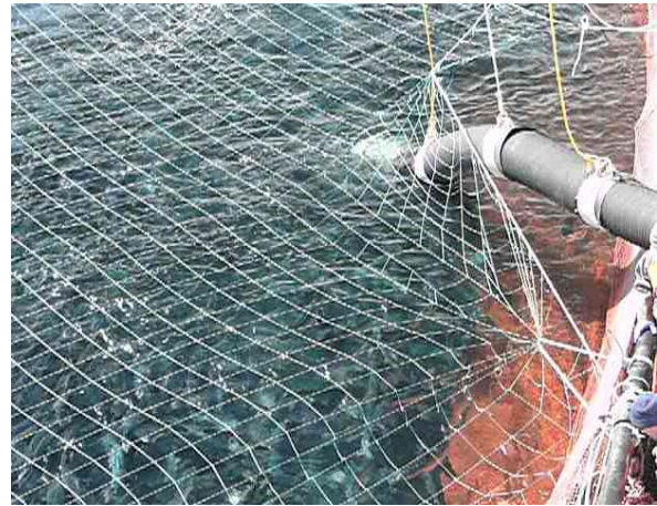
Figure 37: Using a fish pump to harvest a cage – fish are drawn into the pipe and transported in water to the harvest point
